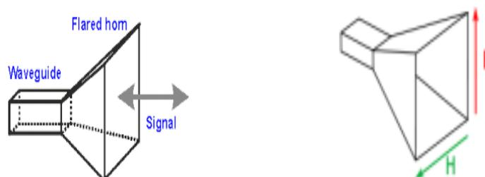
**Fig:** Out structure of Pyramidal Horn antenna
